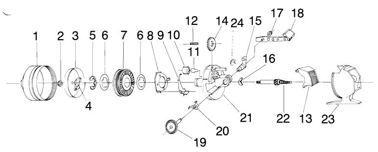
Should the anti-reverse pawl (17) drop out while changing spool, be sure to place back into body assembly with largest flange pointing toward base of reel as shown in diagram. Make sure the arm of the pawl actuator (21) rests in the center of the anti-reverse pawl to reassemble.
